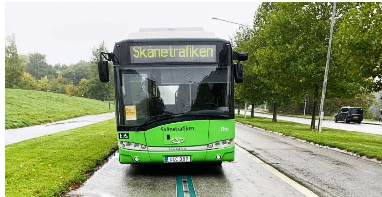
A roughly 21-kilometre stretch of an ERS road feeding an electric bus in southern Sweden (Skania)
